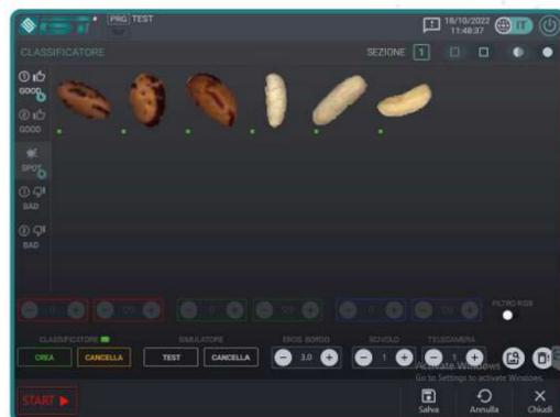
An **internally developed** software intended to allow the operator to manage programs in a fully autonomous way. A self-learning system can be used to set up a program within just a few minutes, which automatically captures images of compliant products and all defects to be discarded.
