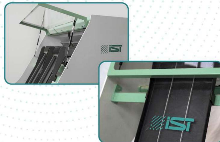
**Vibrating plates with front drop by gravity**, for improved incoming product control. **Chutes with an anodising treatment for use in the food industry** for preventing wear and tear over time, designed to ensure a constant flow over the entire surface. A proprietary **uniform LED lighting** system offering a perfect comprehensive view of the products to be inspected, without loss of quality and without overheating.
